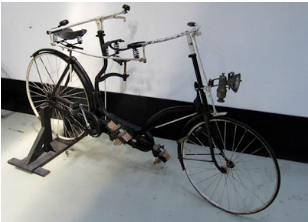
A Danish over 55 tandem for a couple who both want to go the same way. (Notice the two handlebar steering).
