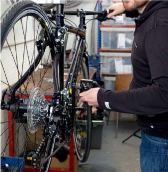
If it is slow to go into the higher gears, screw in the cable adjuster. Re-check that all the securing bolts are tight and go for a gentle test ride.
